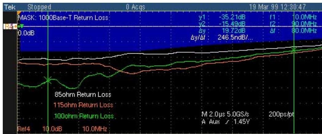
Figure 8-23: Waveform for 1000BASE-T Return Loss
