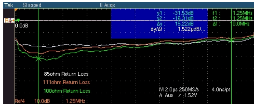
Figure 10-23: Waveform for 10BASE-T Return Loss Transmitter
