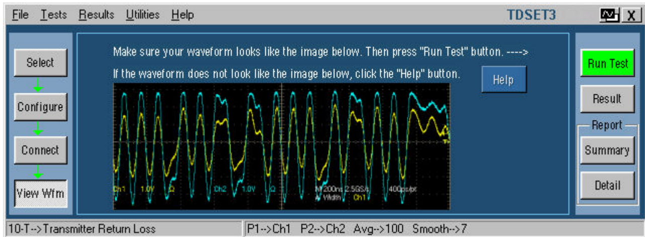
Figure 13-9: 10BASE-T View Waveform for Return Loss
