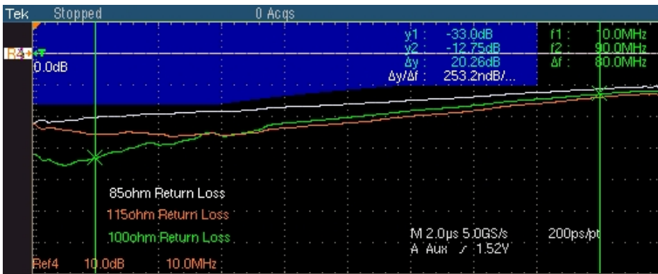
Figure 9-18: Waveform for 100BASE-TX Return Loss Transmitter
