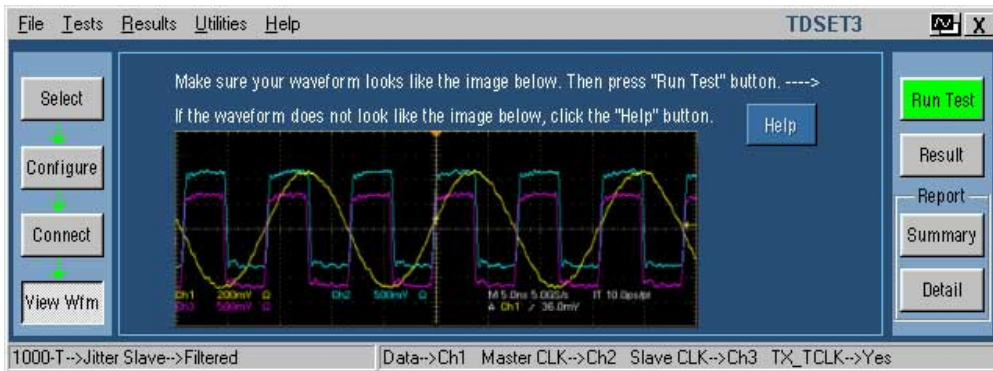
Figure 11-7: 1000BASE-T View Waveform for Jitter Slave Filtered (with TX_TCLK access)
