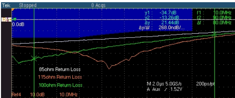
Figure 9-19: Waveform for 100BASE-TX Return Loss Receiver
